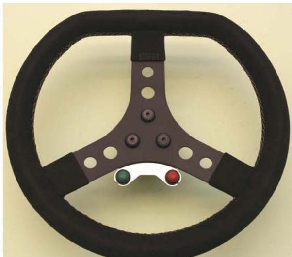
Ensure that the wiring from the push buttons are then cable tied to allow full movement of the steering wheel without causing the wires to chafe. Then connect to the PVL Driver Control Unit via the PVL Extension cable provided located at front of battery mounting bracket. Cable tie as required.
